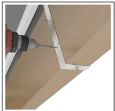
Fix locating straps to rafters/trusses using tech screws.
